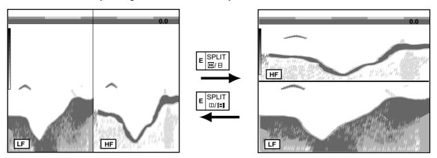
How to use the E:SPLIT soft key (example: dual frequency display)
